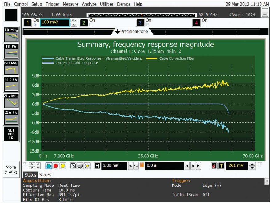
Figure 7. Example of frequency response correction of a cable. The 3dB down point moved from 21 GHz to 62 GHz.
