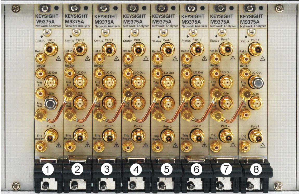
Figure 1-7 Installing Semi-Rigid Cable M9370-20018
