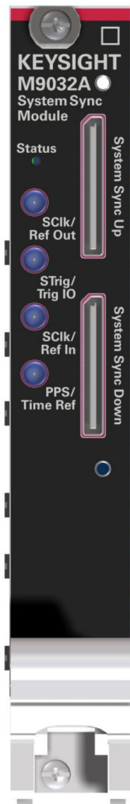
Figure 1 Front view of the M9032A single width 3U PXIe module
