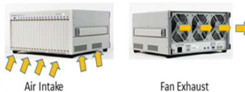
Figure 6 Depiction of air flow in the M9018A chassis
