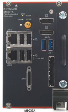
Figure 8 Front panel view of M9037A Embedded Controller
