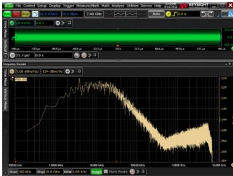
Figure 8: Expected Power Spectrum Density of Alien Cable Bundle Noise
